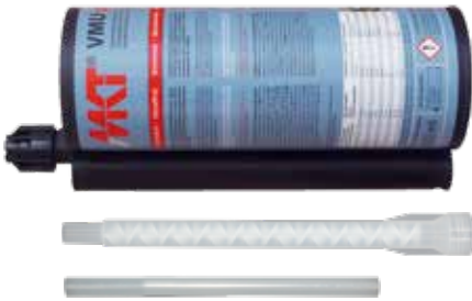
Cartridge VMU plus 825 Side-by-side cartridge Content: 825 ml With big mixer VM-XL and reducer / extension tube for drill holes down to 12mm diameter
